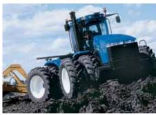
T9000 engines produce from 380 to 480 hp and also give you up to 40% torque rise and power growth of up to 54 hp. That's more than enough power and torque to pull the heaviest carry-all scraper.
